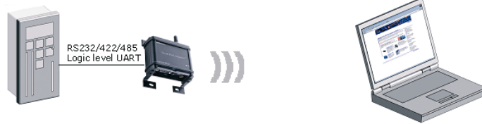
Picture 2. The Serial Port Adapter connected to the controller communicates wirelessly with a Bluetooth enabled Laptop.
